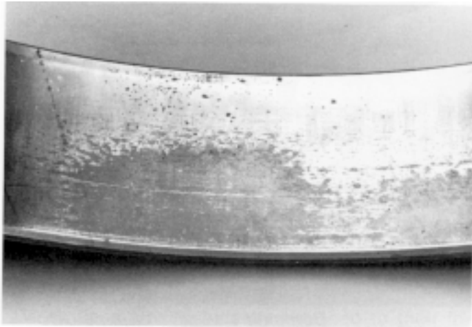
Bearing race "flaking"
