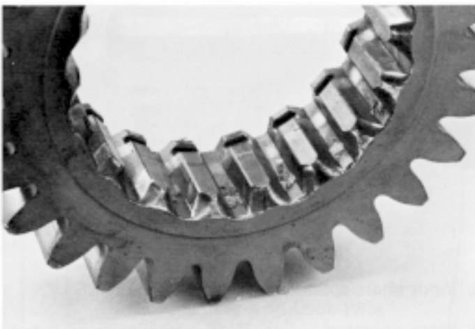
Snubbed clutching teeth
