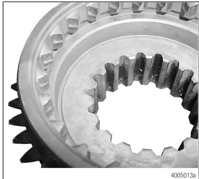
CLUTCHING TEETH DAMAGE DUE TO TORSIONAL VIBRATION
